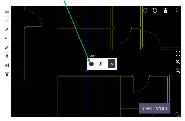
Alternatively, you can create control points after laser alignment.
