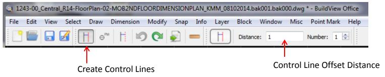
Reference Lines: tap "Reference line", input offset distance, tap on entity to offset, select which side to offset
