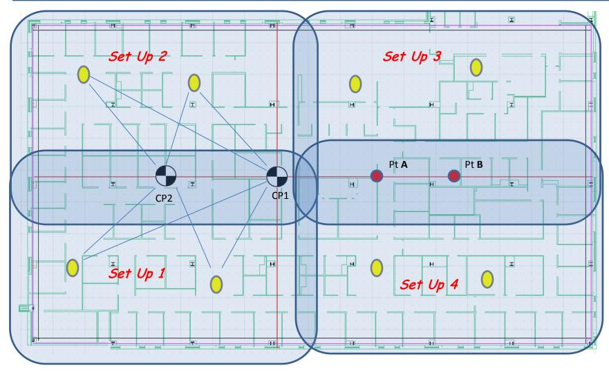
Another option is to use points between 2 Set Ups for more than Set Up. Center control lines were used for CP1 and CP2 and Pt A and Pt B
