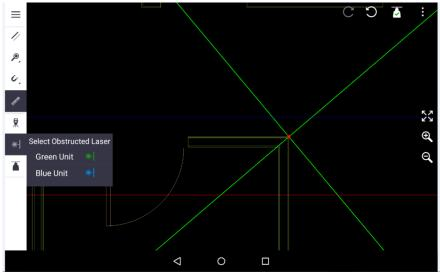
Tap on non Blocked laser to locate new temporary point Distance along non Blocked laser is given. Measure back manually
