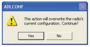
Click **Yes** to copy the default settings from the radio's permanent memory to the computer RAM for review and editing. The radio does not use any changes until you click **Program** in the main dialog or in the *Exit* dialog. When restoring factory defaults, the ADLCONF current channel table is retained.
