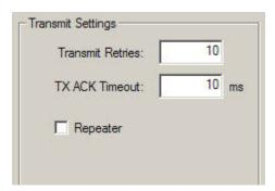
**Note** – Only Transparent EOT/EOC and Packet Switched protocols support transmit retries. So when you select any other protocol (on the Serial Interface screen described on page 21), the Transmit Settings section of the Radio Link screen displays only the Repeater check box.
